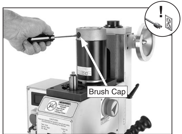
Figure 59. Removing brush cap.
